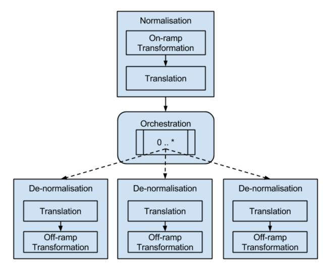
Each mediator should consist of a **normalisation** sub-components, a **orchestration** sub-component and a **de-normalisation** sub-component. The purpose of each of these are described below.
